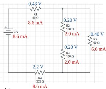
Step 4: The voltages through R1 and R4 are given by Ohm's law
